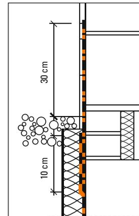
*Application of render or plaster placed directly on the bituminous waterproofing system can lead to cracks occurring in the covering!*
